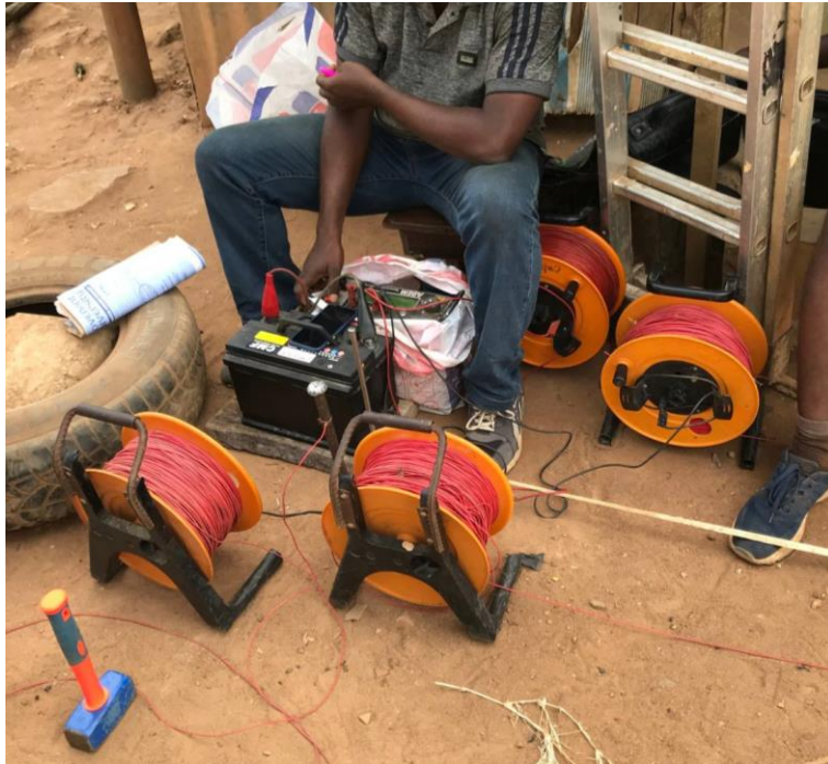
Figure 3.10: Base station set up for ERT traverse Profile 2 (Aduloju street)
