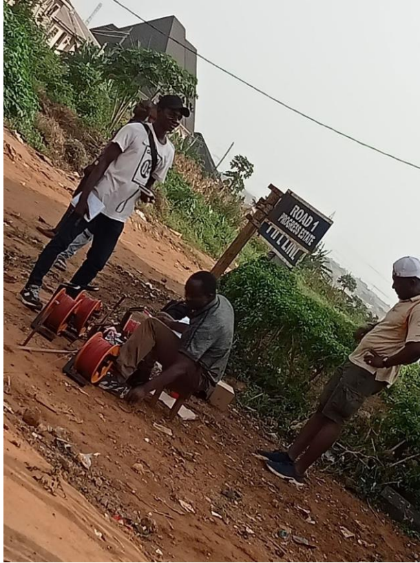
Figure 3.13: Base station set up for VES survey
