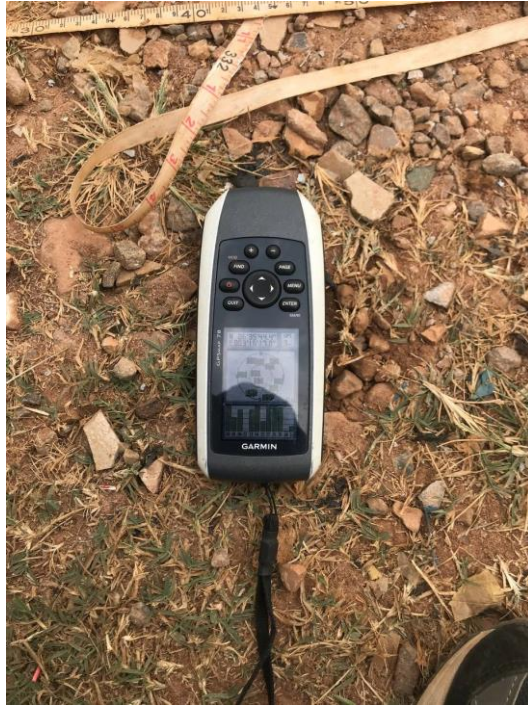
Figure 3.3: Garmin GPSMAP 78 Handheld Marine GPS Device
