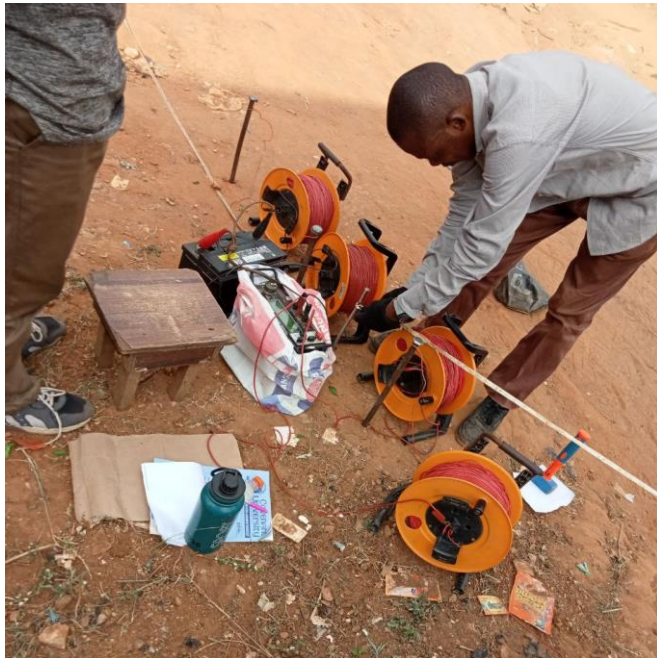
Figure 3.12: Base station set up for ERT traverse profile 3 (Church Street)
