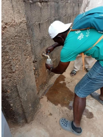
Figure 3.14: Water sample being collected from local resident's tap
