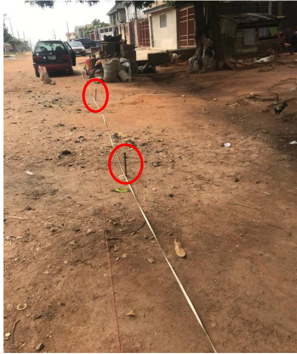
Figure 3.7: ERT traverse for Profile 1 (steel electrode rod indicated by the red circle)
