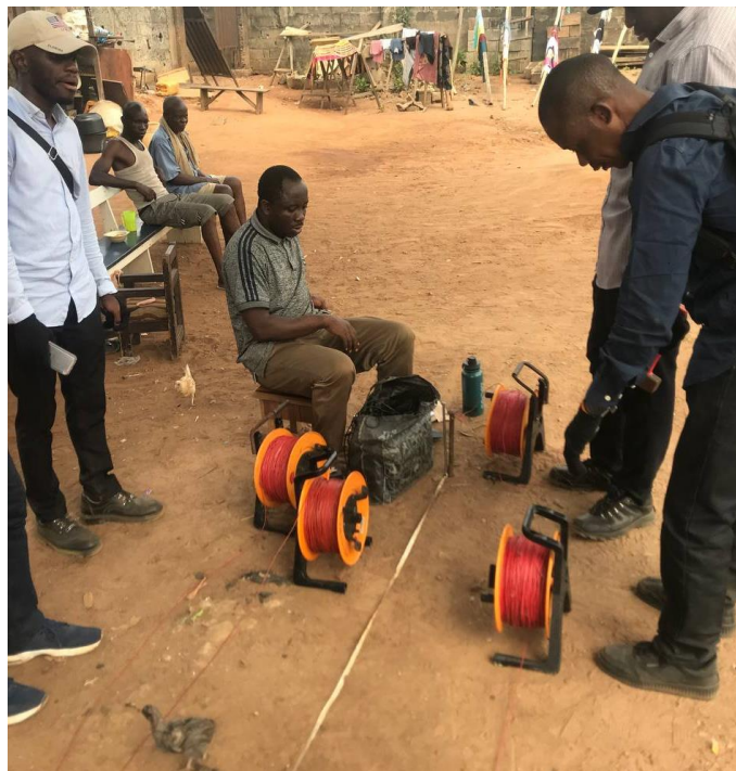
Figure 3.8: Base station set up for ERT Traverse 1 (Road 1)
